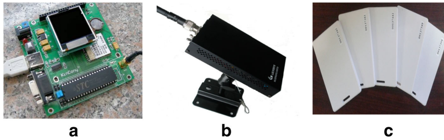
Fig. 1 Tag location device. a Vehicle mounted GNSS; b RFID reader; c RFID tags
